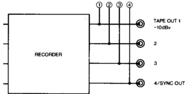
FIGURE 22: all output is at -10 dB.
