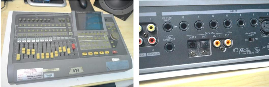
**FIGURE 4: The front panel and its controller; Figure 5 the rear are the sockets for other possible connections (Photographs and all following photographs of the author).**
