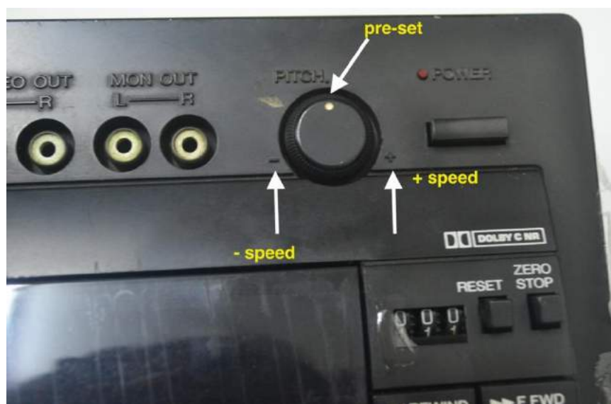
FIGURE 7: Tape speed of the replay unit.
