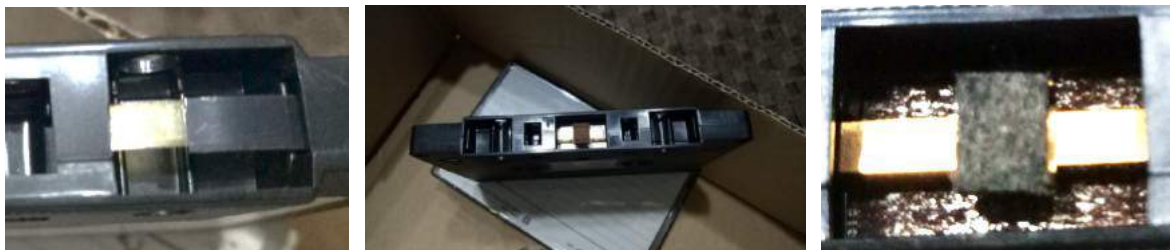
FIGURE 8: Deterioration due to fungus; FIGURE 9a and b: Mechanical issue such as broken tapes, rusted magnetic shield.
