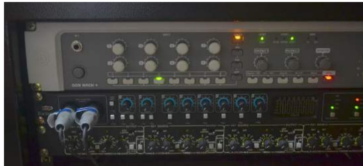
FIGURE 23a and b: Direct RCA outputs – 10dBv to the inputs of audio interface independently.
