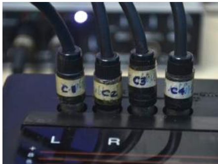
FIGURE 23a and b: Direct RCA outputs – 10dBv to the inputs of audio interface independently.
