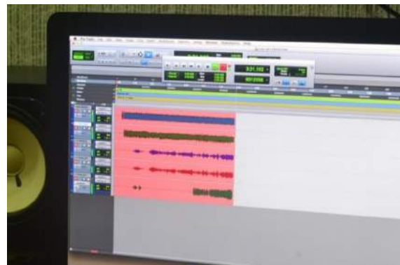
FIGURE 24a and b: Migration of audio signal (real-time) from the replay unit of independent outputs to the direct inputs of the Digital Audio Workstation with the bit resolution and sampling rate recommended by the IASA-TC04.
