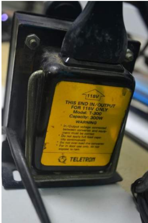
FIGURE 11a and b: Transformer from 220 volts to 115 volts.
