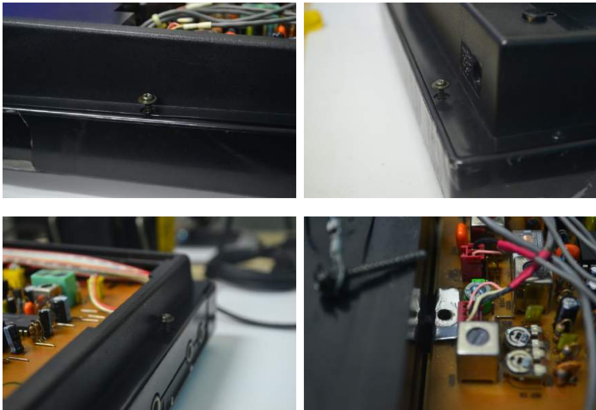
FIGURE 13a, b, c, and d: Four screws have to be removed, with the last being attached to grounding of the circuit board.
