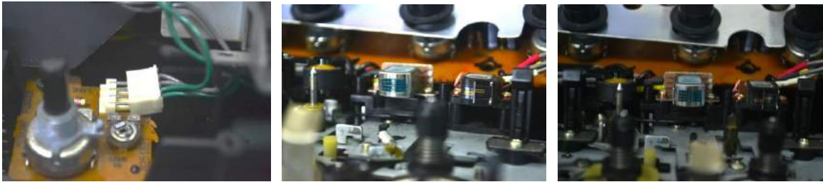
FIGURE 17, 18: Removal of the variable speed control switch. FIGURE 19: Azimuth and Zenith adjustments for clearer sound quality.
