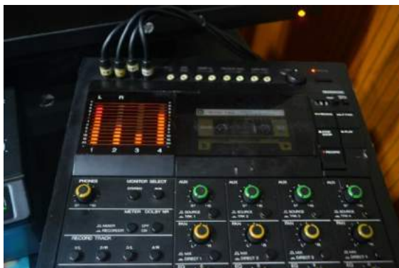
FIGURE 24a and b: Migration of audio signal (real-time) from the replay unit of independent outputs to the direct inputs of the Digital Audio Workstation with the bit resolution and sampling rate recommended by the IASA-TC04.
