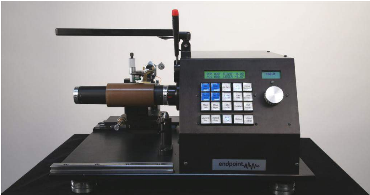
FIGURE 2: Wax cylinder replay and digitization equipment in the "endpoint audio lab" (photo by the author).
